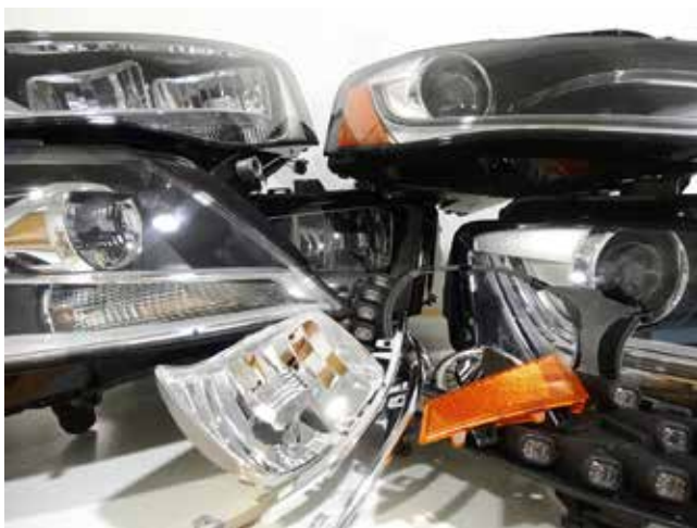
Fig. 1. Mixed waste from headlight production: fully assembled headlights (left), and aluminum-coated plastics (right) (© Fraunhofer IVV)
