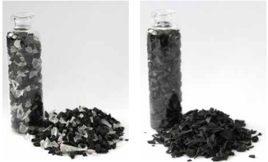
Fig. 6. Exemplary plastic fractions with purities >90% after automatic sorting: PC fraction (left), PP fraction (right). For optimum comparability, the material was shredded after fractioning
