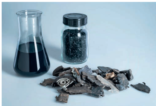
Fig. 2. Foreground: shredded feedstock, back left: polymer in solution, back right: compounded pellets of post consumer recycle (PCR). © Audi AG
